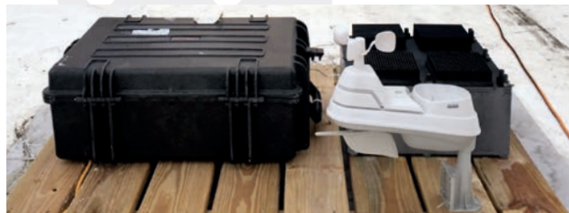
The team’s test device, which has been deployed on the roof of an MIT building for several months, was used to prove the principle behind their new energy-harvesting concept. The test device is the black box at right, behind a weather-monitoring system (white) and a set of test equipment to monitor the device’s performance (larger black case at left).
